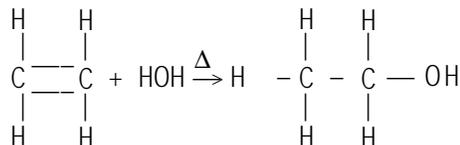
Ethylene + Water → Ethyl Alcohol
